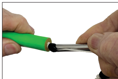
Step 3: Push the bridle approximately 1cm into the gun rubber.
