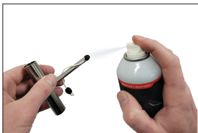
Step 2: Lubricate the dyneema bridle bead.
